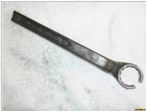
Box end 7/8" with a section cut out to clear the wire. 2)
