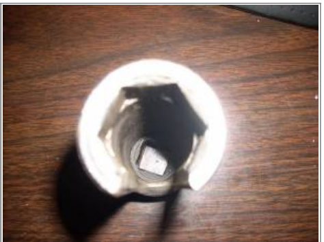
7/8" deep well 6 point socket with a side milled out to clear the wire 3)
