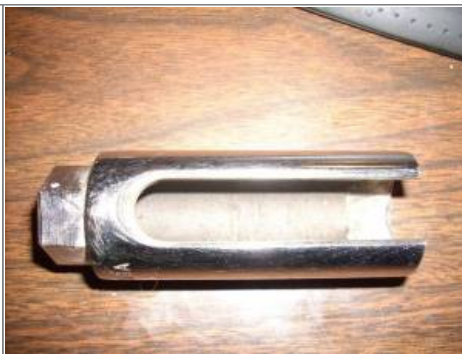
7/8" deep well 6 point socket with a side milled out to clear the wire 3)
