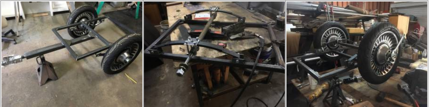
Home made pull - behind trailer with motorcycle wheels 1)
