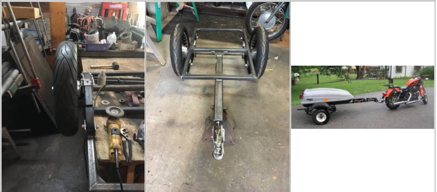
Home made pull - behind trailer with motorcycle wheels 2)
