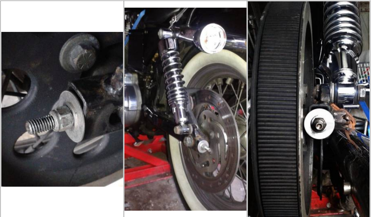
One large fender washer with a smaller one in front to keep the large one from bending. 15)
