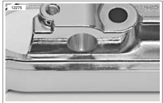
Figure 3. New Chrome Inner Rocker Cover (No Slots) (Part No. 17537-96C) Introduced 9/12/05
