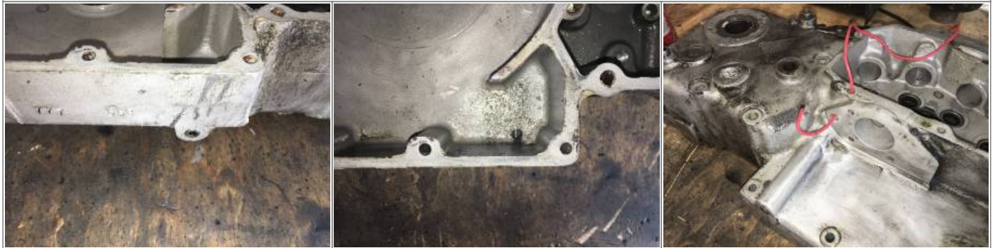
Scavenge passage on 77 engines 28)
