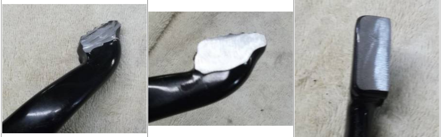
Pedal fitted to mark the hole location. The hole was drilled with a 17/64" bit, and then threaded with a 5/16"-24 tap. (same bolt that comes with the Trap Shift Peg, or the same thread as used on the shifter) This hole could have been drilled straight through with a nut on the end of the bolt but this way looks cleaner. 4)
